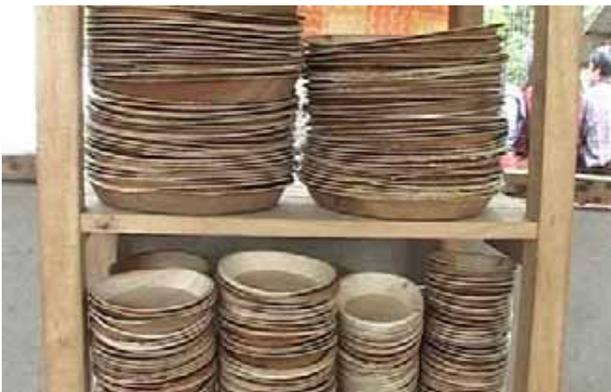
The plates are made from cleaned and dried sheaths of betel nut trees which are pressed into moulds of various sizes and designs. The three machines currently in operation can produce about 600 plates a day. The SNV's Representative said that while this is a promising venture, maintaining quality, reliability and price would be important if they were to expand the market. The project is also expected to benefit Sherzong, Umling and Taraythang, which have large areas of betel nut plantation.
