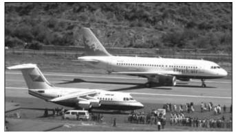
One of Druk Air's new Airbus 319s, with the old BAe 146 in the foreground. The Airbuses have greater capacity and range.
